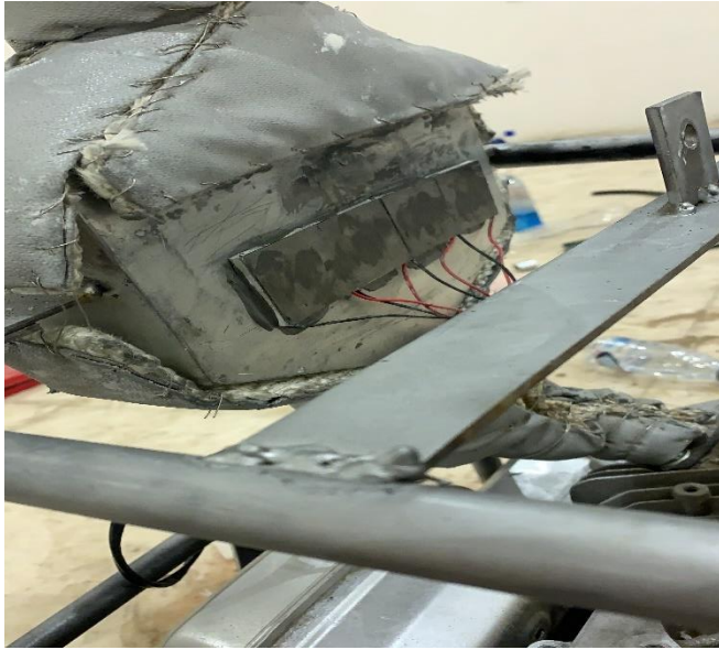
TEG connection in parallel
