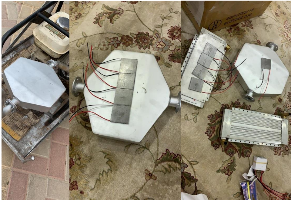
Figure 20: a) Actual system from which waste heat to be recovered. b) Installation of thermoelectric generators on top and bottom surfaces of heat exchanger. c) Heat sink installation on top and bottom surfaces.
