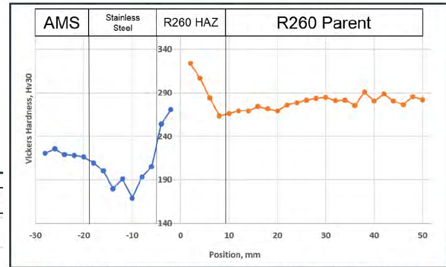
Figure 10: Hv30 hardness trace across AMS, Stainless Steel and R260 metals
