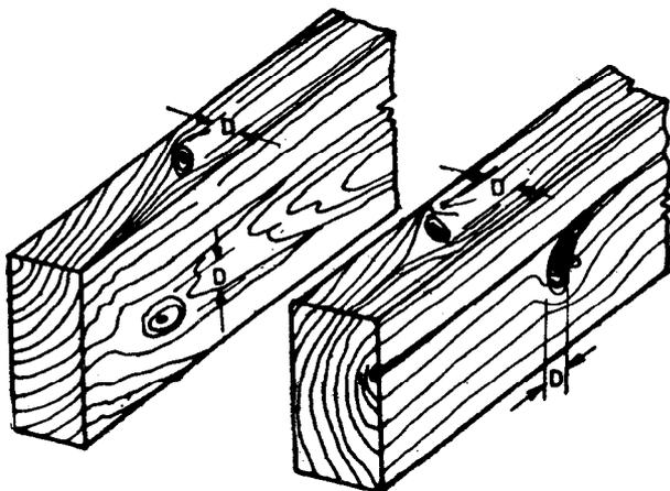
FIG. 2 MEASUREMENT OF KNOTS IN BEAMS
