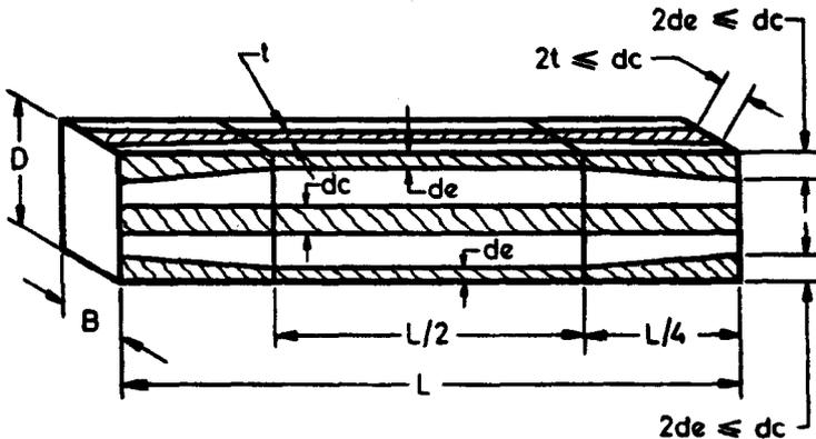
$dc$  = Maximum size of the allowable knot in centre line of the wider face ( allowable size to be determined by grading rules ).
