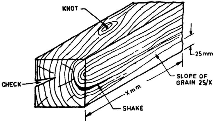
FIG. 1 KNOTS, CHECKS, SHAKES, AND SLOPE OF GRAINS
