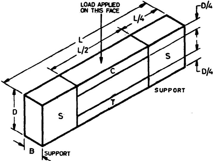
Zone of critical tension ( $T$ ), compression ( $C$ ), and shear ( $S$ ). The allowable sizes, numbers, etc., of the strength reducing defects such as knots, for any particular grade of timber, are generally worked out with respect to these zones.
