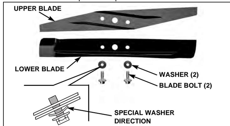
8. Tighten the blade bolts with a torque wrench. Wear thick leather gloves and hold the blades with your hand to prevent the blades from turning when tightening the bolts, as shown on page 13.
