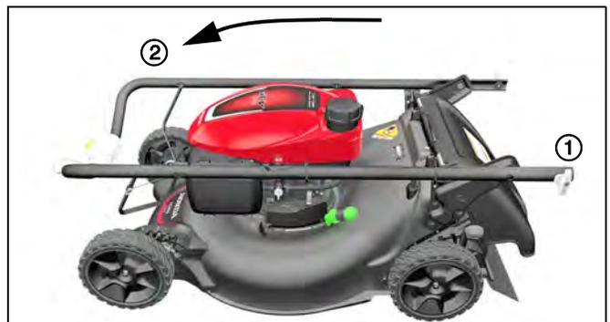
1. Turn the handlebar adjust knobs 90 degrees to release the locating pins ①.
