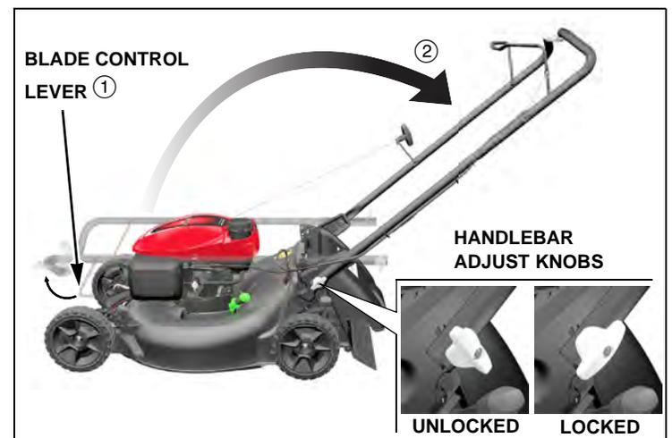
2. Align the adjust knobs with one of the two holes on each handlebar stay. Setting the adjust knobs in the lowest holes raises the handlebar to its highest position.
