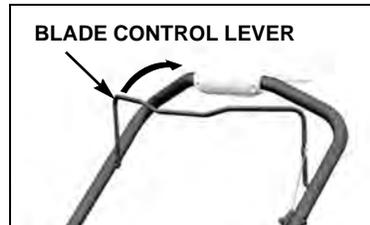
Continue to hold the lever fully against the handlebar. This will keep the engine and blades rotating smoothly and prevent premature wear to the flywheel brake system.
