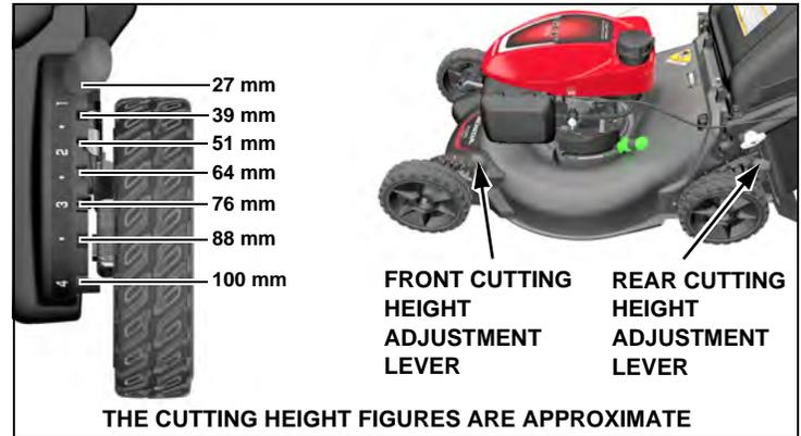
If you are not sure what cutting height to select, start with a high setting and check the appearance of the lawn after mowing a small area. Then readjust the cutting height if necessary. Refer to the "Mowing Tips" on [page 9](#) for additional cutting height recommendations.
