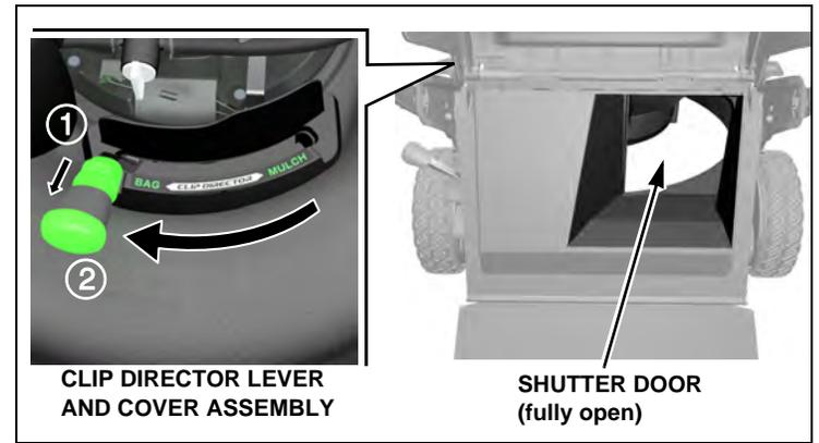
To discharge clippings to the rear, remove the grass bag and leave the Clip Director lever in the BAG position.
