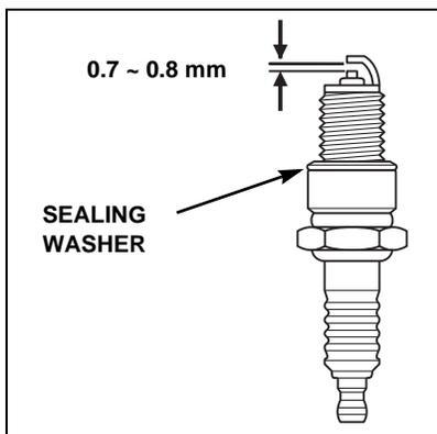
If reinstalling the old spark plug, tighten 1/8 to 1/4 turn after the spark plug seats.
