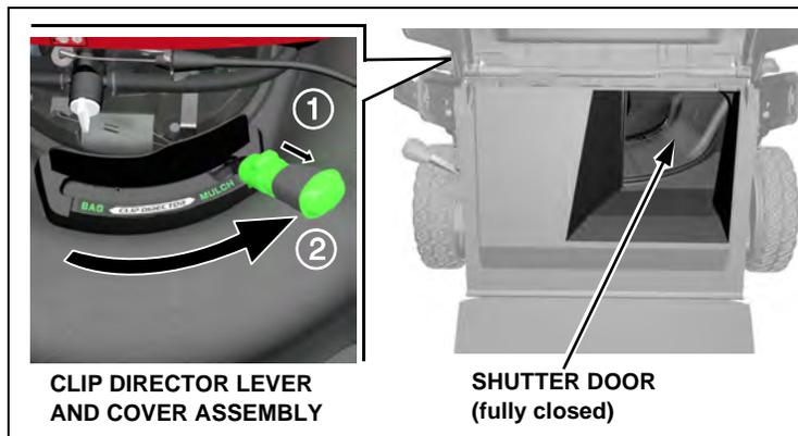
Some grass accumulation in the discharge opening is normal when the Clip Director is in the MULCH position. To remove this grass, close the discharge guard, set the Clip Director to the BAG position, engage the blade control lever, and start the engine.
