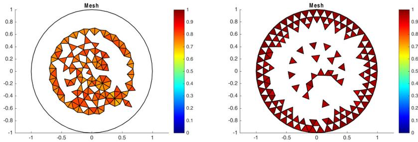
Figure 3-17: Visualizations of the mesh quality: worst 25% (left) and best 25% (right).
