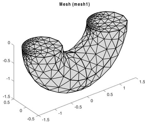
Figure 3-14: Free tetrahedral mesh after the use of the CopyFace feature.
