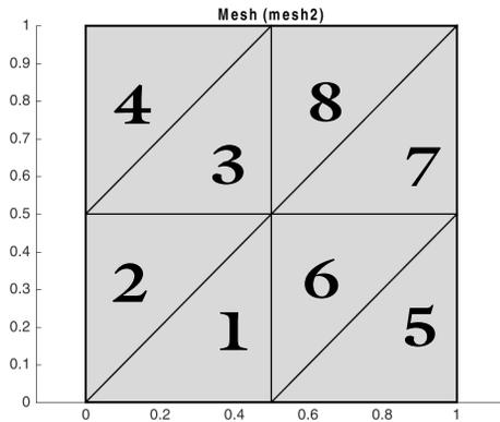
*Figure 3-18: Mesh with elements (bold) and nodes (italic) indices.*
