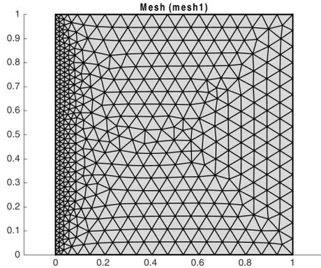
Figure 3-3: Refined mesh on boundary 1 (maximum element size = 0.02).
