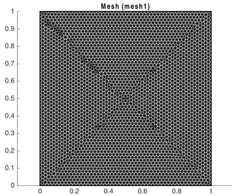
*Figure 3-2: Fine mesh (maximum element size = 0.02).*
