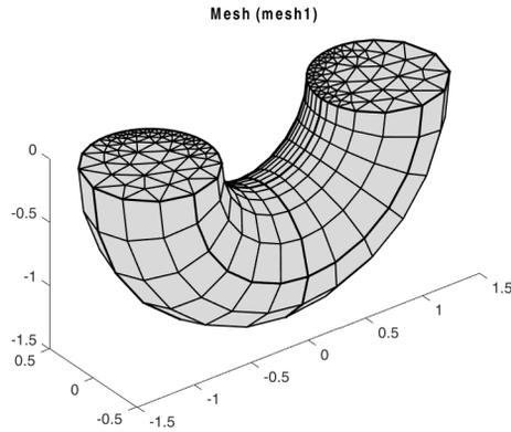
*Figure 3-13: Prism element obtained with the CopyFace and Sweep features.*
