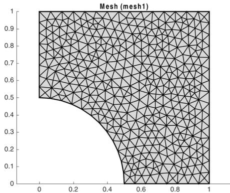
*Figure 3-4: Mesh created with the Delaunay method.*
